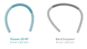
Image showing deployed balloon in silicone tubing at 14 atm.<sup>3</sup>
